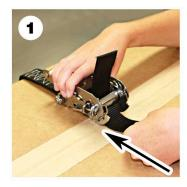
To thread ratchet buckle, place the long unattached strap end THROUGH slot in center of closed ratchet.
