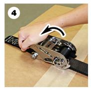
4. Webbing will wind itself and be locked in place so that further ratcheting will rapidly increase tension in strap. Close ratchet fully when finished.
