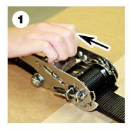
To release webbing, pull and hold release tab on top assembly to override ratcheting function.
