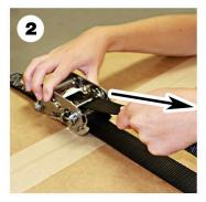
Pull attachment side of webbing through the slot. There must be a minumum length of 1"-inch for assembly to function properly.
