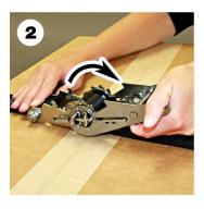
Open ratchet until it is flat and both assemblies are in-line. The top assembly will click into place and hold open.
